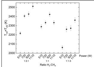
Fig. 1. H<sub>2</sub> rovibrational temperatures in microwavedriven mixed hydrogen/methane plasma at 50 mbar
